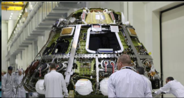
Thermal cycle test completed on Orion crew module
