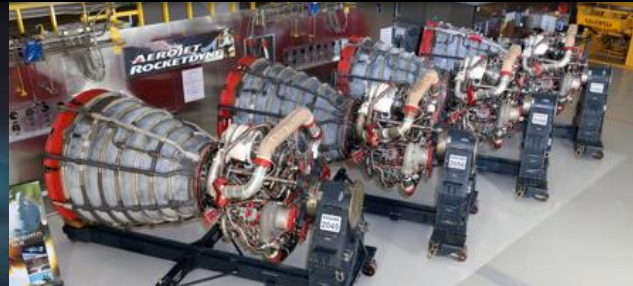
The four RS-25 engines that will power SLS
