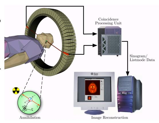
Positron emission tomography (PET) uses Fluorine-18, half life of ~110 min
