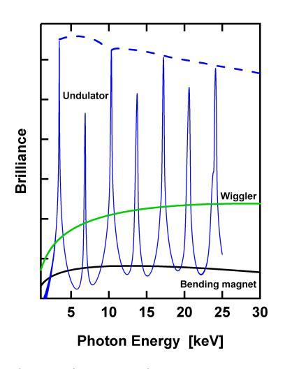
Produced in synchrotron radiation sources using bending magnets, undulators and wigglers
