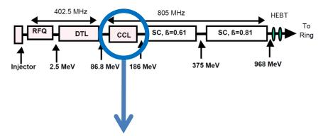
4 modules, each containing 12 accelerator segments CCL and 11 bridge couplers. The CCL section is a RF Linac, operating at **805 MHz** that accelerates the beam **from 87 to 186 MeV** and has a physical installed length of slightly over **55 meters.**
