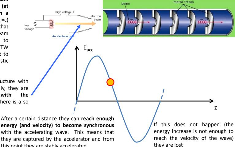
energy (and velocity) to become synchronous with the accelerating wave. This means that they are captured by the accelerator and from this point they are stably accelerated.
