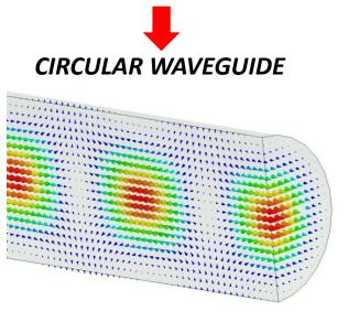
As example if we consider a simple circular waveguide the first propagating mode with  $E_z \neq 0$  is the TM<sub>01</sub> mode. Nevertheless by solving the wave equation it turns out that an e.m. wave propagating in this **constant cross section waveguide** will **never be synchronous with a particle beam** since the **phase velocity is always larger than the speed of light c**.
