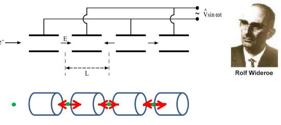
$\Rightarrow$ If the **length of the tubes** increases with the particle velocity during the acceleration such that the time of flight is kept constant and equal to half of the RF period, the particles are subject to a **synchronous accelerating voltage** and experience an energy gain of  $\Delta E = q \Delta V$  at each gap crossing.
