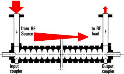
It is possible to demonstrate that, in order to keep the accelerating field constant along the structure, the iris apertures have to decrease along the structure.
