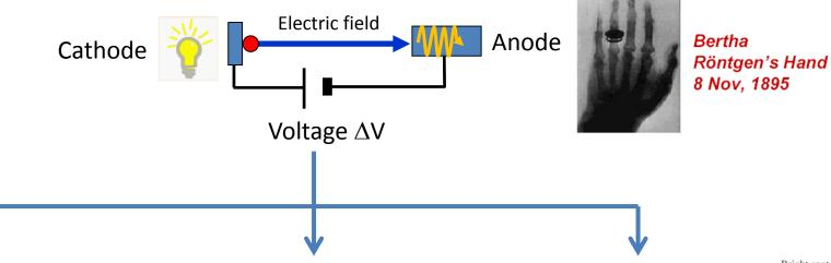
The **energy gained** by the electrons travelling from the cathode to the anode is equal to their charge multiplied the DC voltage between the two electrodes.
