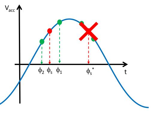
$\Rightarrow$ The choice of the synchronous phase in the positive slope of the RF voltage provides longitudinal focusing of the beam: **phase stability principle**.
