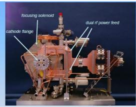
Solenoids field are used to compensate the space charge effects in low energy guns. The configuration is shown in the picture
