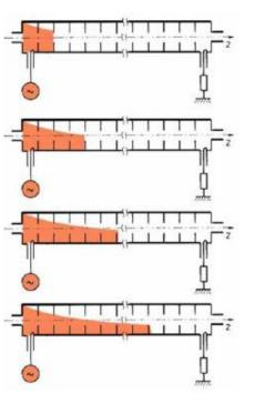
In a purely periodic structure, made by a sequence of **identical cells** (also called "**constant impedance structure**"), the RF power flux and the intensity of the accelerating field decay exponentially along the structure :
