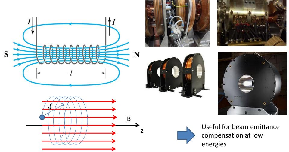
Particles that enter into a solenoidal field with a transverse component of the velocity (divergence) start to **spiralize describing circular trajectories**.
