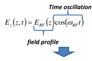
$\Rightarrow$ There is another possibility to accelerate particles: using a **travelling wave (TW)** structure in which the RF wave is **co-propagating** with the beam with a **phase velocity equal to the beam velocity**.
