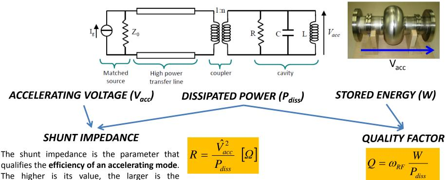
The higher is its value, the larger is the obtainable accelerating voltage for a given power. Traditionally, it is the quantity to optimize in order to maximize the accelerating field for a given dissipated power:
