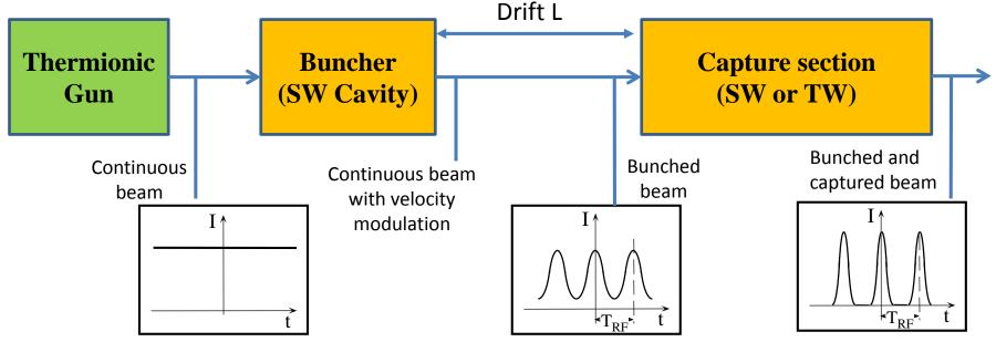
$\Rightarrow$ Bunching is obtained by modulating the energy (and therefore the velocity) of a continuous beam using the longitudinal E-field of a SW cavity. After a certain drift space the velocity modulation is converted in a density charge modulation. The density modulation depletes the regions corresponding to injection phase values incompatible with the capture process
