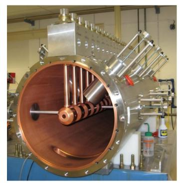
CERN LINAC 4: 352 MHz frequency, Tank diameter 500 mm, 3 resonators (tanks), Length 19 m, 120 Drift Tubes, Energy: 3 MeV to 50 MeV,  $\beta$ =0.08 to 0.31  $\rightarrow$  cell length from 68mm to 264mm.
