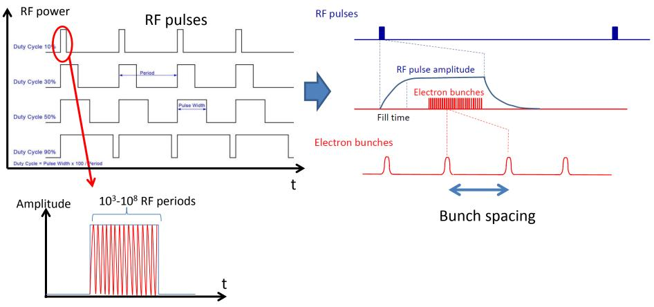
$\Rightarrow$ Because of the very low power dissipation and low RF power required to achieve a certain accelerating voltage the SC structures allow operation at very high Duty Cycle (DC) up to a CW operation with high gradient (>20 MV/m).
