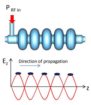
Is equivalent to the superposition of two counterpropagating TW waves
