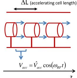
The energy gain per cell (one gap + tube in case of a DTL) of a generic particle and of a synchronous particle are (we put  $\theta$ =0 in the generic expression of the accelerating voltage just for simplicity ):
