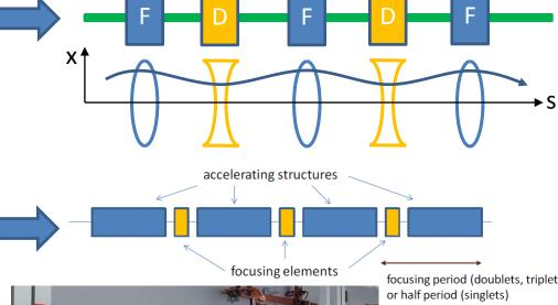
$\Rightarrow$ The type of magnetic configuration and magnets depend type/distance on the type of particles/energies/beam parameters we want to achieve.
