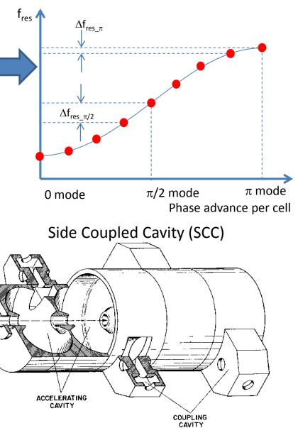
$f_{\text{RF}}\text{=}800$  - 3000 MHz for proton ( $\beta\text{=}0.5\text{-}1\text{)}$  and electrons
