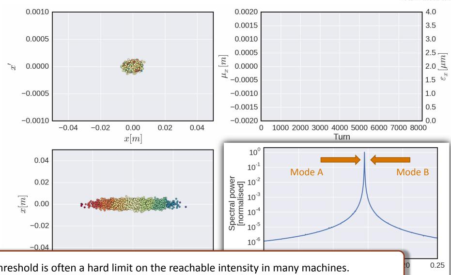
The TMCI threshold is often a hard limit on the reachable intensity in many machines.
