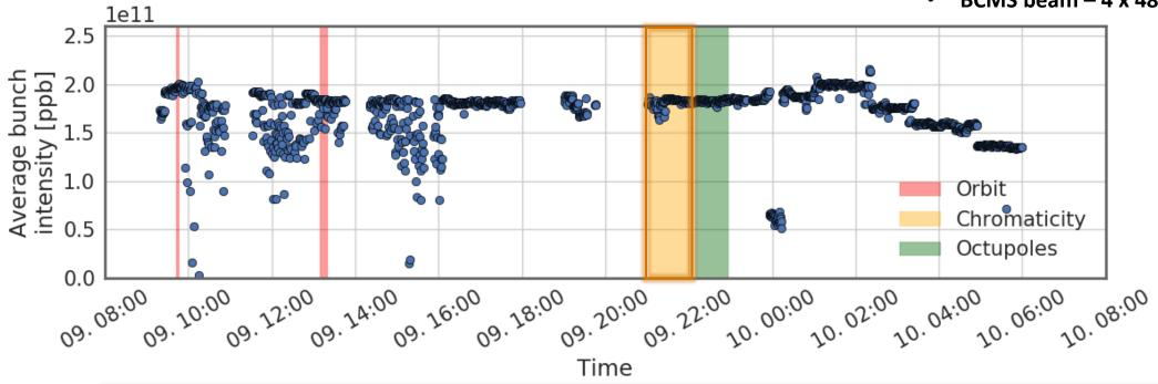
The horizontal coupled bunch instability at 20 MHz did no longer appear with the transverse damper now having been fine adjusted resulting in finite gain at these frequencies.
