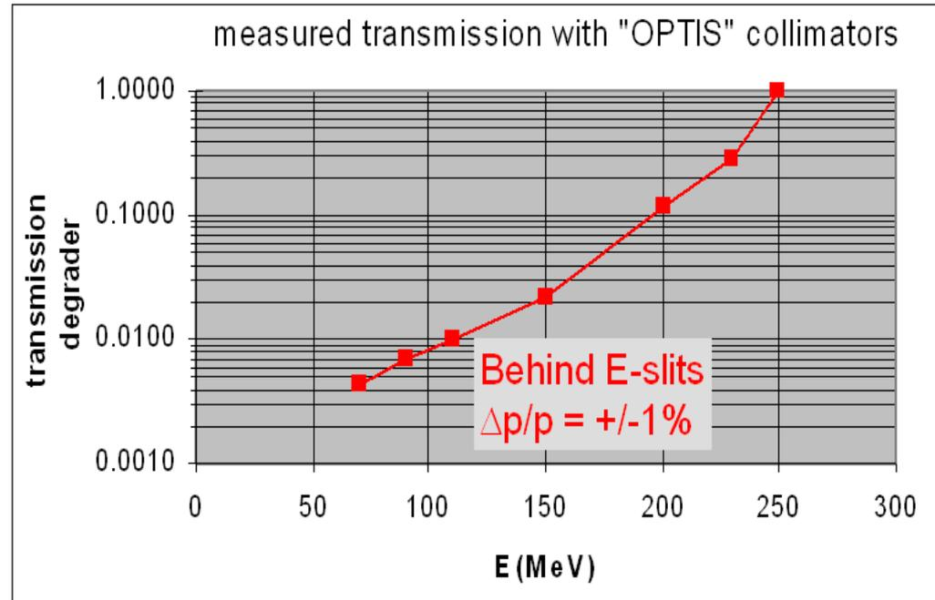
degrader: (carbon wedges in vacuum) and laminated beam line magnets for fast energy changes < 80 ms / step
