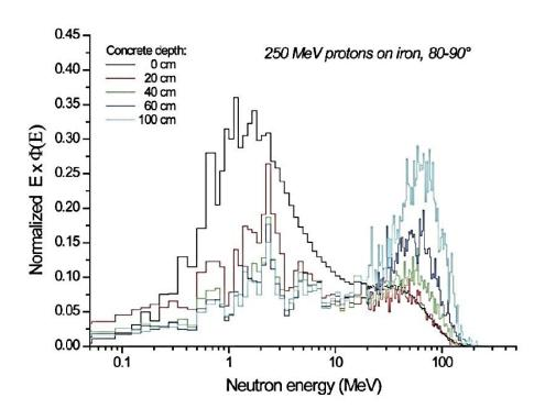
Fig. 6: Neutron energy distributions  $E\Phi(E)$  in the transverse direction generated by 250 MeV protons impinging on an iron target thicker than the proton range. The distributions are for source neutrons and behind concrete shields of thicknesses ranging from 20 cm to 1 m. The distributions have been normalized to unit area in order to show better the change in the shape of the spectrum with increasing shield thickness.
