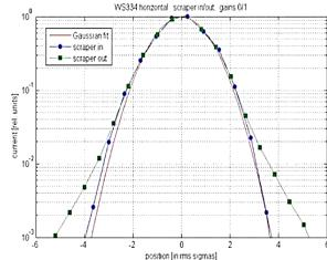
Example: SNS LINAC Scraping at 3 MeV profile measurement at 40 MeV M. Plum, CERN-2016-002
