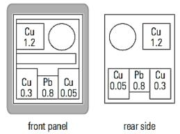
(thickness of filters in mm)
