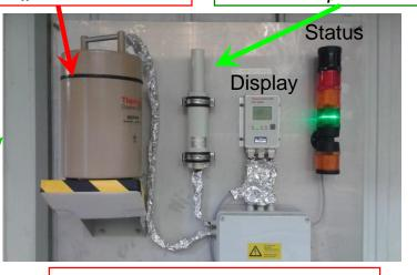
Moderated thermo-luminescence detector for passive n-detection
