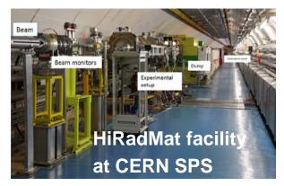
**Beam:** 440 GeV  $\approx 10^{13}$  protons,  $\sigma_x = \sigma_y \approx 2$  mm within  $t = 50 \mu s$   $\Rightarrow E_{tot} \approx 1 \text{ MJ}$
