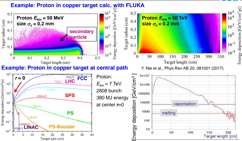
**Remark:** Low energetic proton have large energy deposition at short range e.g.  $E_{kin} = 50 \text{ MeV}$
