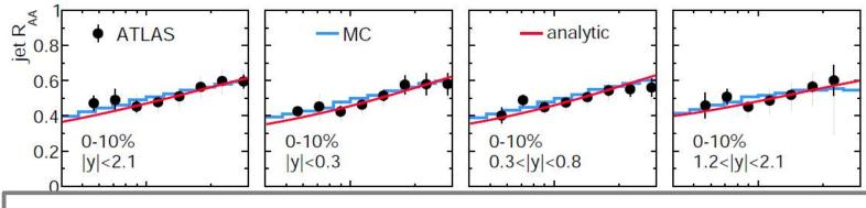
–> Flatness and no rapidity dependence of jet R<sub>AA</sub> can be explained as a consequence of different energy loss of quark and gluon initiated jets on top of steeply falling p<sub>T</sub> spectra of initial partons
