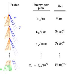
will decrease in terms of number of particle. The depth at which both components reach critical energy is also where the number of particles in the shower reaches maximum. This depth is called  $X_p^{max}$  and the number of particles at that point is called  $N^{max}$  (also called the shower size).
