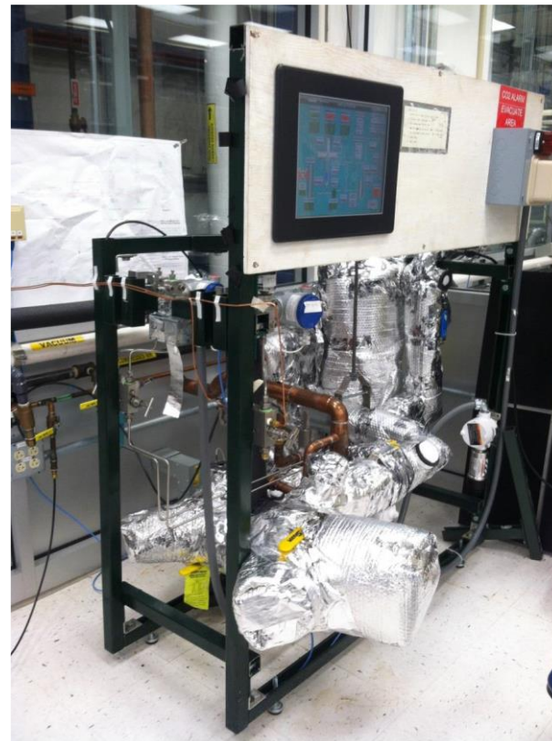
CO 2 cooling plant at FNAL
