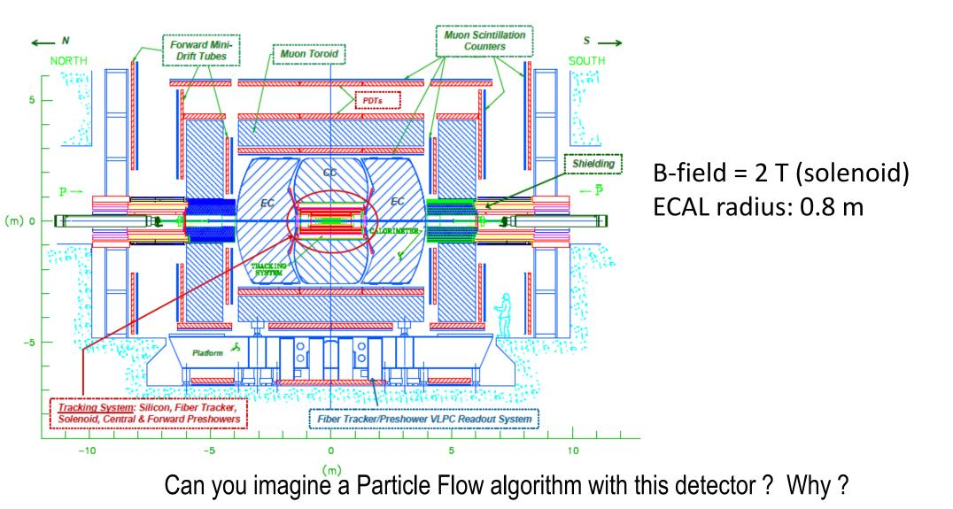
The B-field integral is small (2x0.8)=1.6 T.m (to be compared to ~5 for CMS !) There is material in front the calorimeter (2 X0 at normal incidence) Granularity of both tracking and calorimeters are not sufficient, given the particle rates at ppbar colliders. "Energy flow" technics were tried but were not successful enough to become standard.
