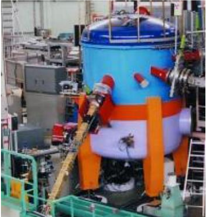
Turbine with counter rotating blades to decelerate the neutrons
