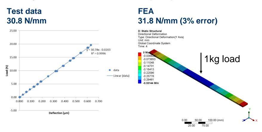
NOTE: we always also do a similarly-sized aluminum beam in the test and FEA to validate the overall methodolgy
