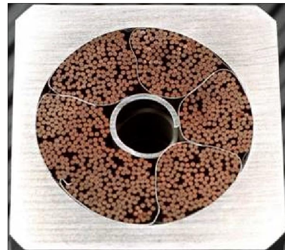
~1152 wires ITER Nb 3 Sn cable
