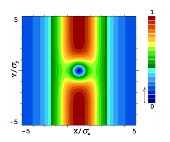
Due to the crossing angle, particles traverse the opposite bunch horizontally.
