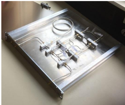
Fig 2. Proof of concept filter installed in rack box.
