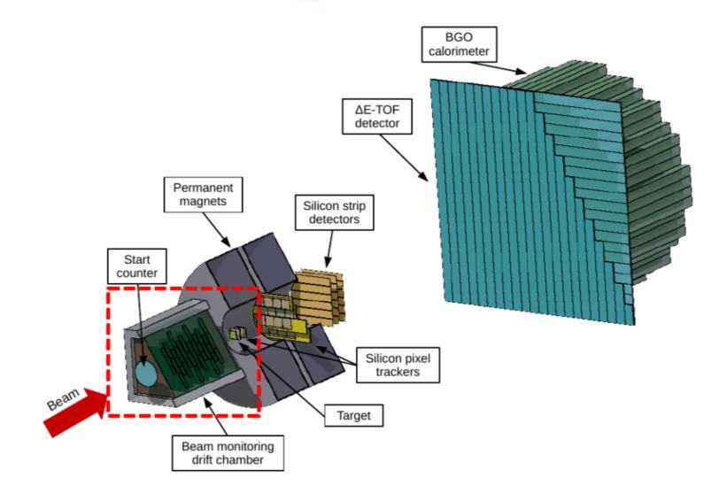
Drift chamber of 11 cm x 11 cm x 20 cm dimension composed of 12 orthogonal layers of wires.
