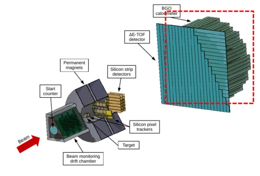
BGO calorimeter with 20 cm radius (344 pixels)  $2 \times 2$  cm pitch (same as the  $\Delta$ E/TOF).
