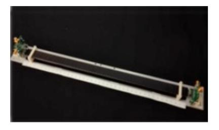
Plastic scintillator wall composed of two layers of bars read-out by SiPMs
