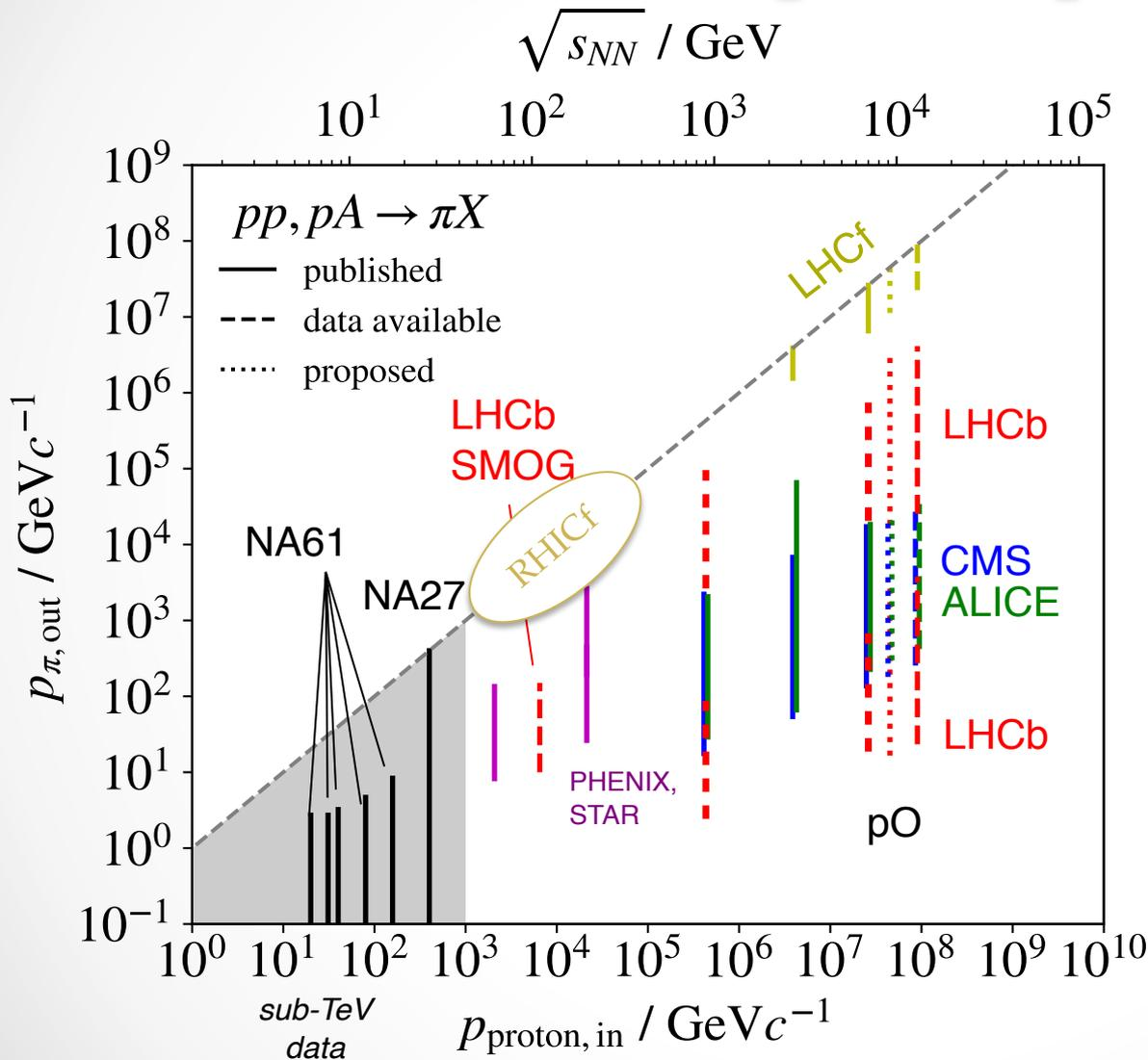
Phase space of air shower interactions as covered by various experiments (beam-beam collisions transformed to equivalent fixed-target system)
