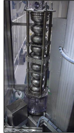
Vertical test High pressure rinsing
