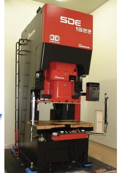
Servo press machine (AMADA, Japan) Max. applying force: 1500 kN
