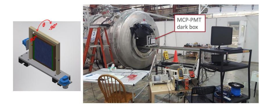
(left) Self-designed test stand with the capability of testing MCP-PMTs up to 20 x 20 cm<sup>2</sup> (right) Picture of MCP-PMT magnetic field test setup at ANL in building 366.
