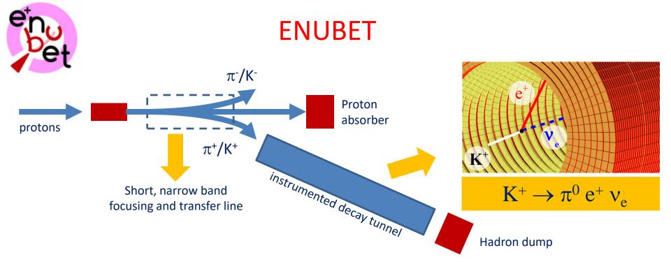
Goal: demonstrate the technical feasibility and physics performance of a neutrino beam where **lepton production at large angles is monitored at single particle level**  $\Rightarrow$  direct measurement of the flux
