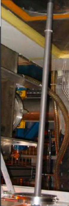
90 cm T2K replica target
