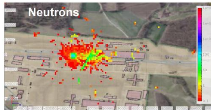
Figure 2: Top view of the ambient dose equivalent (prompt) 10 m above the ground level due to neutrons in \mu\text{Sv/y} .
