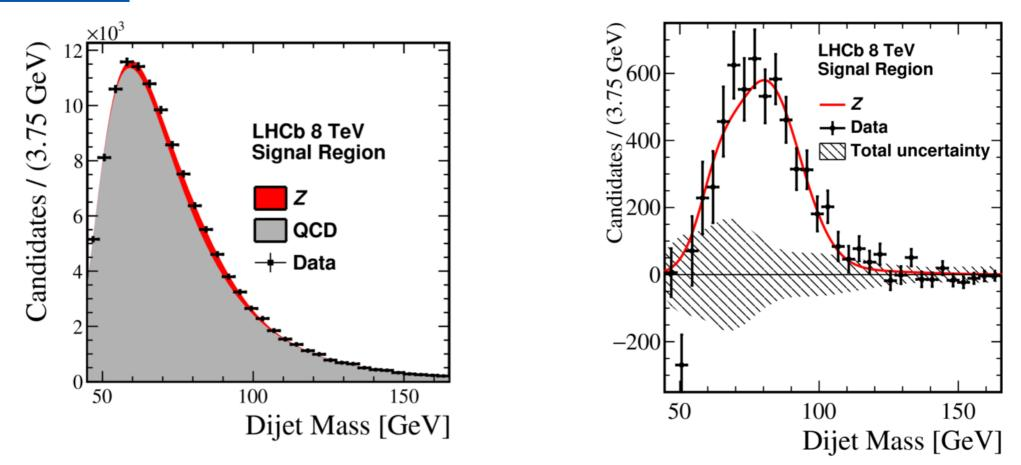
$Z \rightarrow b\overline{b}$  peaks at ~80 GeV: radiation outside of the jet cone, missing energy, asymmetric jet energy resolution.
