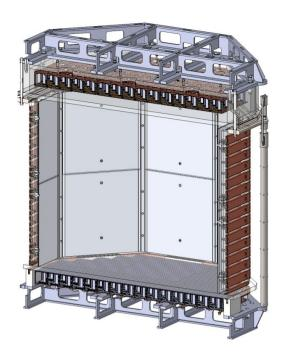
Development of a 1 tonne DS-20k Prototype (CERN -> LNGS), for testing of the cryogenics, electronics, inner components. Possibility for competitive low-WIMP mass search.
