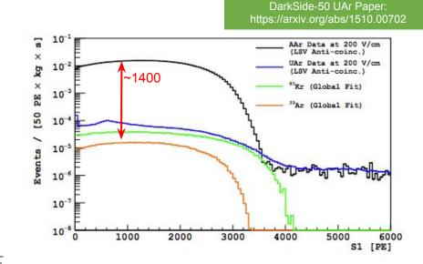
Underground Argon ~1400 reduction in <sup>39</sup>Ar activity. This was demonstrated with DarkSide-50. Argon was extracted in Colorado USA.
