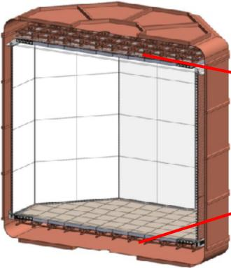
~8000 SiPM Module for Light Readout (Self-production) <u>Crucial</u>: selection of low-radioactive material.
