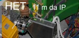
Scintillator hodoscope +PMTs
