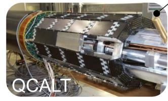
Inner Tracker – 4 layers of Cylindrical GEM detectors Improve track and vtx reconstr.
