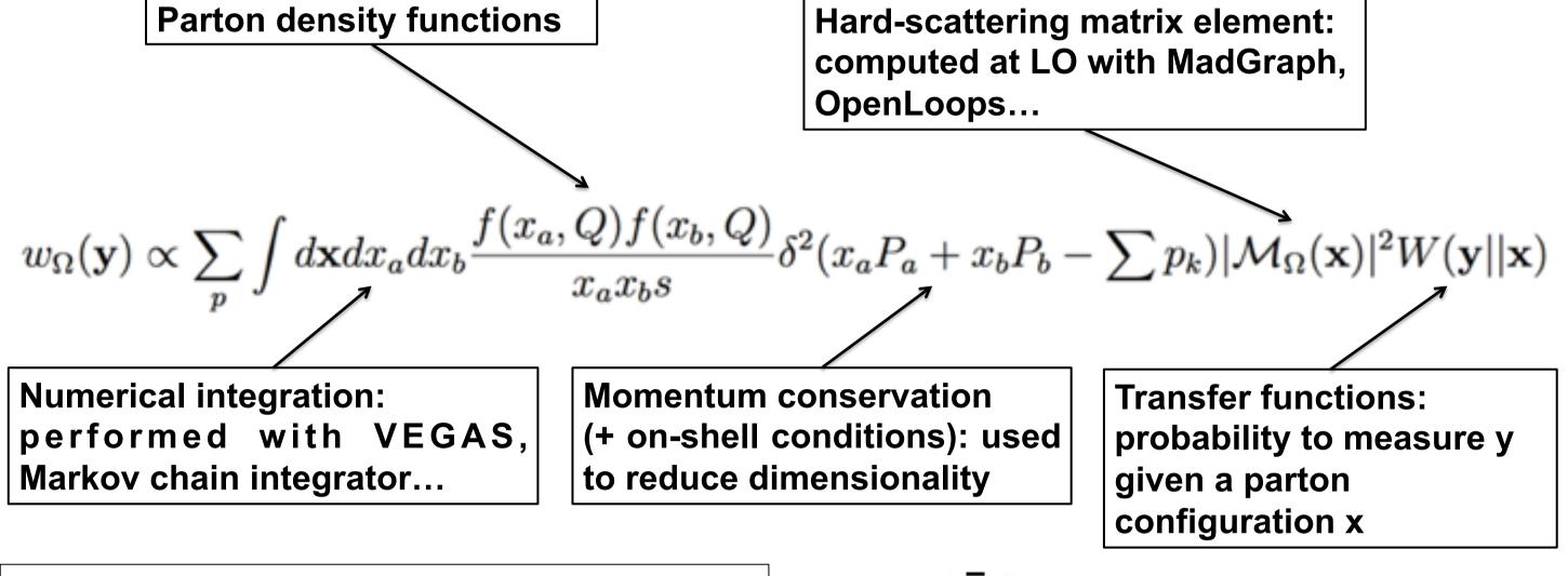
The MEM: The event weight is computed for each hypothesis  $\Omega$  ( $\Omega$ =ttH, ttV...) using observables y as inputs and integrating over unmeasured (or poorly measured) quantities x. The final discriminant corresponds to:
