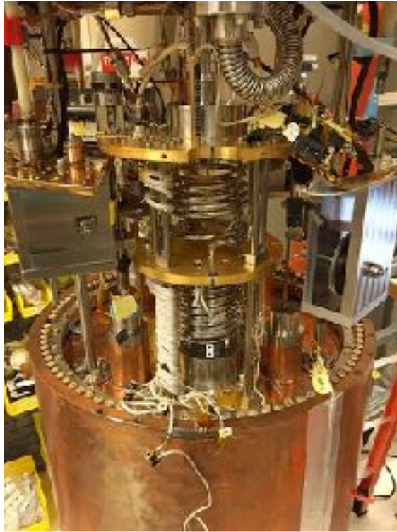
Dilution Refrigerator installed above ADMX Cavity
