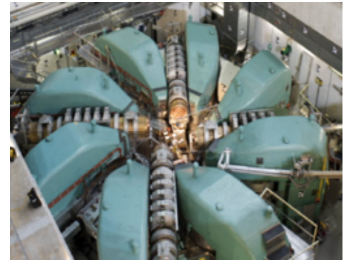
PSI Ring Cyclotron 590MeV, 1.4MW
