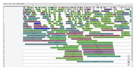
Breakup of operations by CPU core (32-core Xeon).
