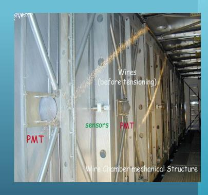
Very good particle ID, energy resolution and "bubble chamber like" picture Of the interaction. Technique developing very fast and promising for large Scale detectors
