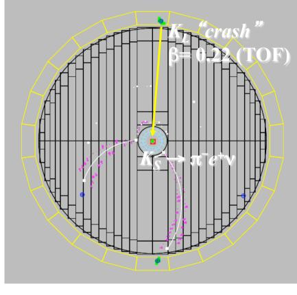
$K_S$  tagged by  $K_L$  interaction in EmC Efficiency ~ 30% (largely geometrical)
