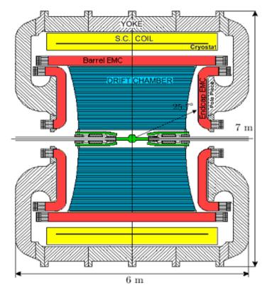
Lead/scintillating fiber calorimeter drift chamber 4 m diameter × 3.3 m length helium based gas mixture
