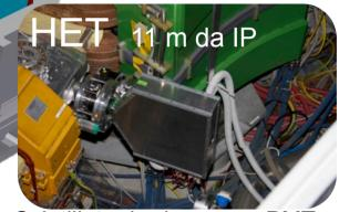
Scintillator hodoscope +PMTs
