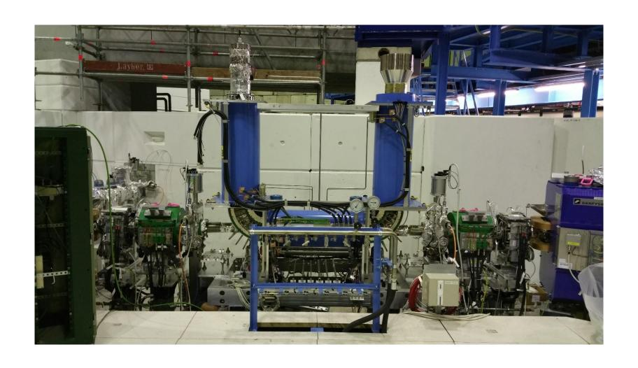
After alignment the vacuum system is closed up Alignment not absolute but to valves.
