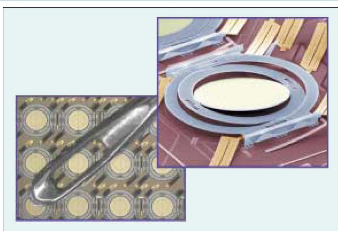
**Figure 4.** Two images of MEMS-based OXC mirrors used in the Lucent LambdaRouter. The image in the upper right is a single mirror, and an array of mirrors is shown in the lower left. An eye of a needle is shown for comparison on the array.
