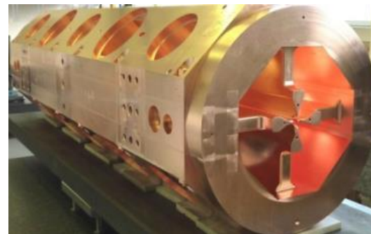
The CERN Linac4 RFQ, 0.05 to 3 MeV, 3 m.
