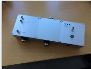
DAQ module to check the performance of the micro-switches, the holding coils and fast opening coils.
