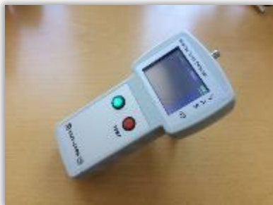
Holding coil inter-turns short checker
