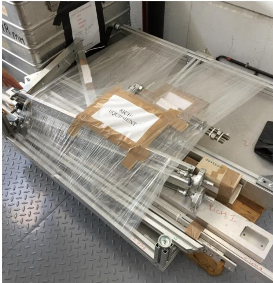
Figure 13 - Old RICH1 Exit Window Installation Toolkit
