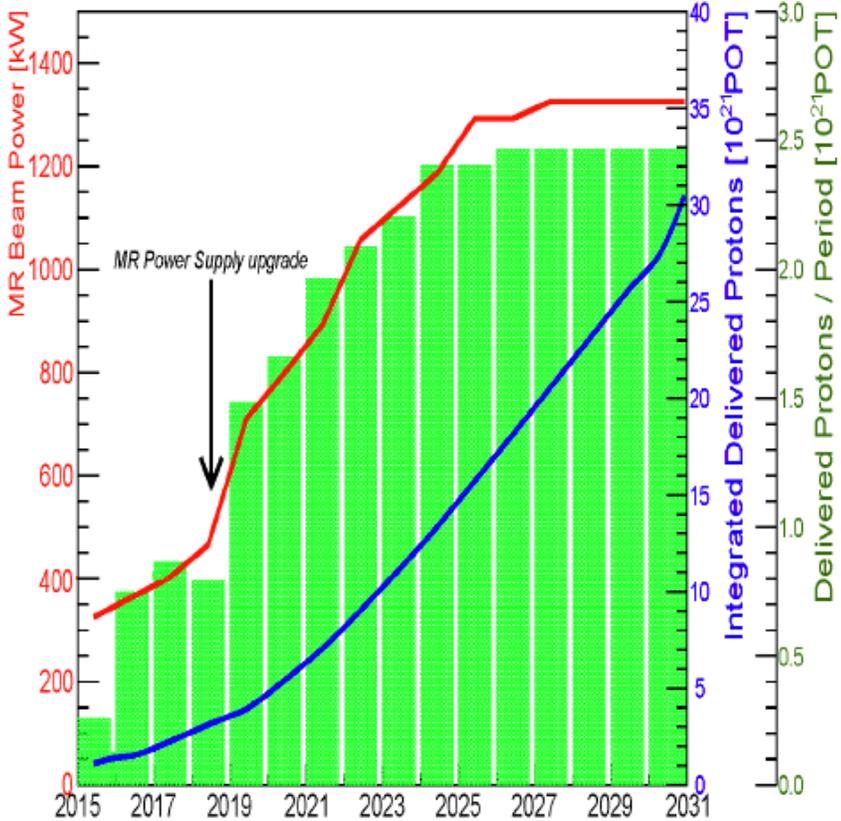
Beam power increase from 500 kW to 1.3 MW
