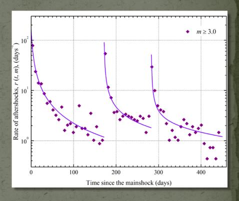
$$r(\geq m_c, t) = \frac{1}{\tau_1 (1 + t/c_1)^{p_1}} + \frac{H(t - t_2)}{\tau_2 \left[1 + (t - t_2)/c_2\right]^{p_2}} + \frac{H(t - t_3)}{\tau_3 \left[1 + (t - t_3)/c_3\right]^{p_3}}$$
