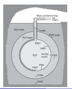
There are many sample points to chose from to gain an accurate representation of the background levels inside the detector.
