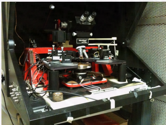
Karl Seuss PSM6 Manual Probe Station
