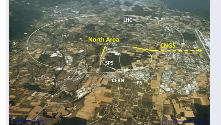
NA62 is the latest generation kaon experiment at the CERN SPS. The experiment is located in CERN in the North Area and extracts protons from the SPS accelerator at 650 GeV/c.
