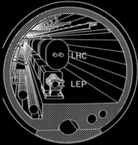
LARGE HADRON COLLIDER IN THE LEP TUNNEL
