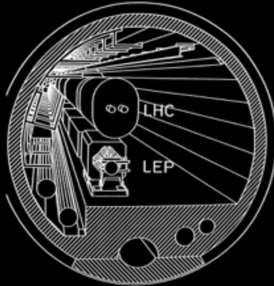
LARGE HADRON COLLIDER IN THE LEP TUNNEL
