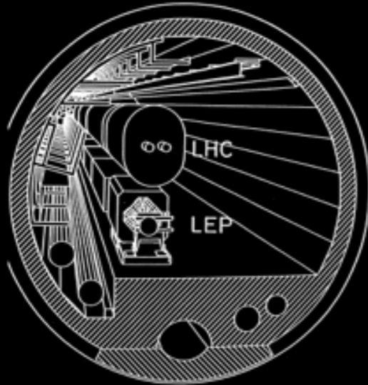
LARGE HADRON COLLIDER IN THE LEP TUNNEL
