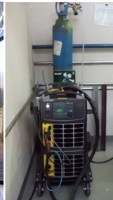
Tungsten Inert gas (Ar) welding with SS 316L
