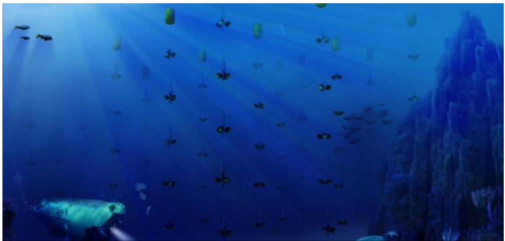
Artist's representation of the ANTARES neutrino detector, made up of 12 strings of photomultipliers that detect and amplify the light emitted by charged particles produced by rare neutrino interactions. [ANTARES]
