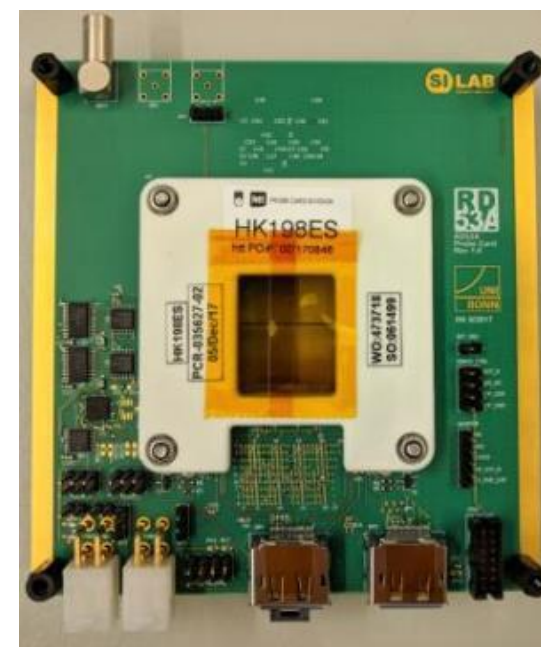
Needle card for wafer probing (developed in Bonn)
