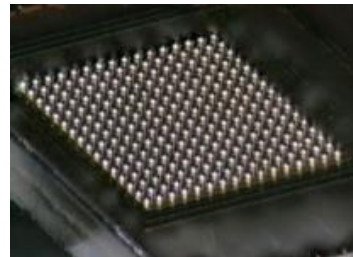
30- \mu\text{m} SAC solder spheres by using the laser-assisted jetting technique
