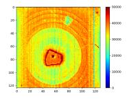
Airy pattern of the zone plate at 1.2 keV can be seen Sensor was damaged with direct beam before this measurement
