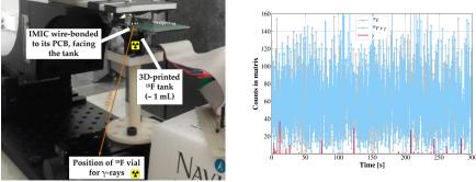
Experiment illustrates the small sensitivity of IMIC to  $\gamma\text{-rays}$  with respect to  $\beta+$
