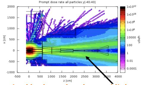
Magnetized hadron absorber and light weight active muon shield to minimize punch through in decay volume
