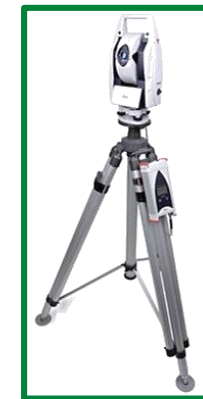
Laser Tracker (Angles and distances measurements)
