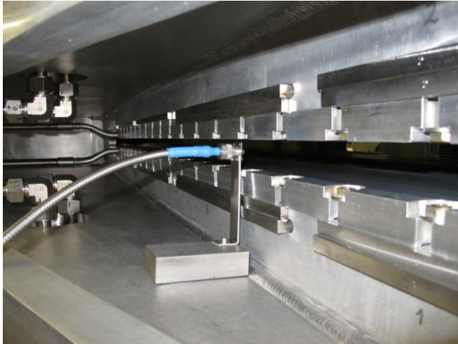
Capacitive pickup in resonator wing to measure the rf radiation out of the beam slit
